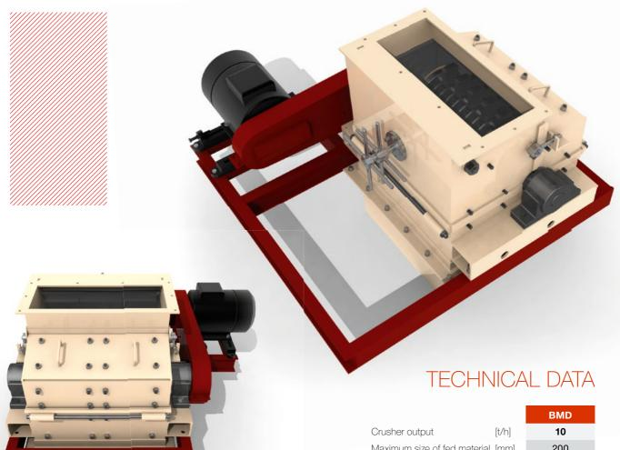
Hammer crusher type 750x260 is designed for crushing of piece-material. The crushing principle consists in bumping of material with a hammer against an impact board. The crushing process proceeds automatically:
