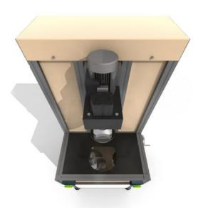
The machine is designed for upper edge soft grinding of thin-walled glass products. It is equipped with a clamping head and two grinding units with flat diamond discs.
